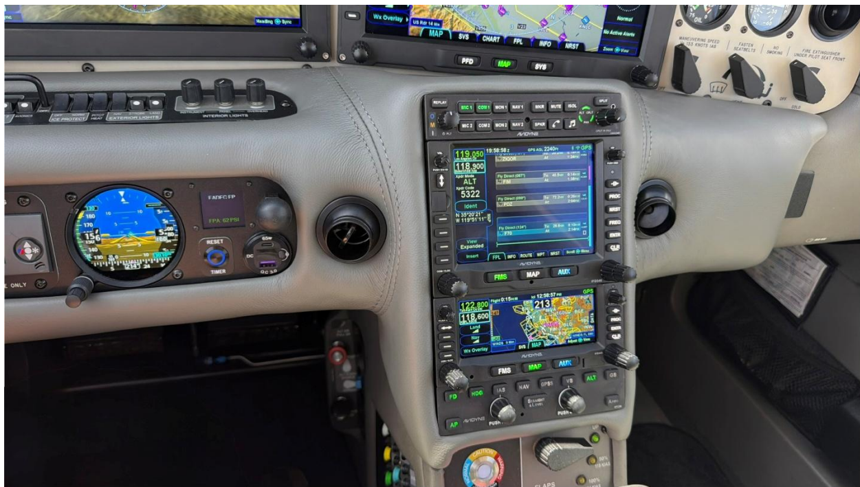
Figure 15: G1 with G3 Surround Installed
