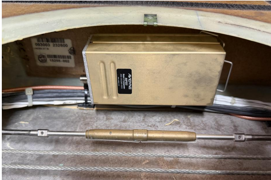
Figure 7: AXP322 Mounting Location in a G3
