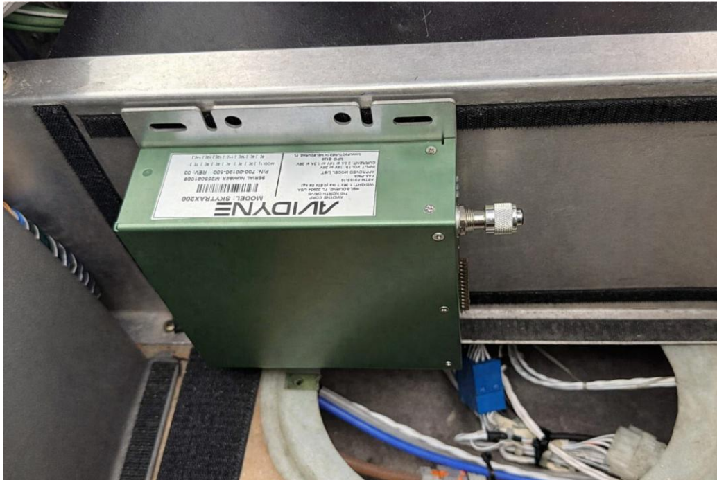
Figure 6: Skytrax Mounting Location on Skywatch 497 Plate
