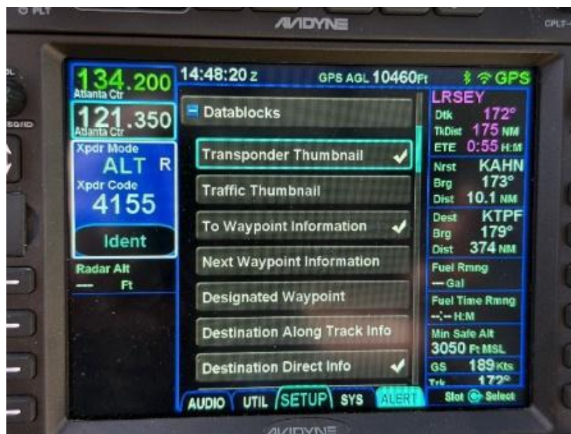
Figure 10: IFD 5XX Transponder Data Block Configuration
