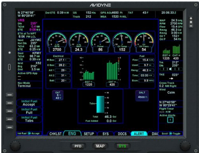
Figure 11 Avidyne Vantage12 700-00212-110 Multi-Function Display
