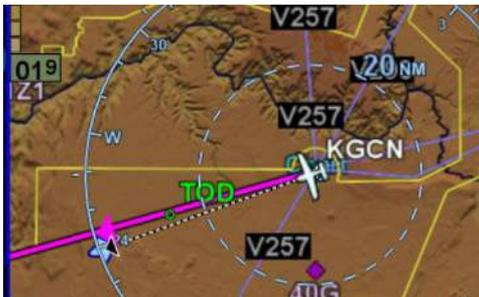
When a target vertical speed is specified, the IFD will compute the TOD point using current groundspeed and the desired descent rate. However, when the aircraft reaches the TOD point and enroute VNAV is allowed, the IFD will compute the angle required to reach the desired altitude, then commence with enroute VNAV using that angle.
