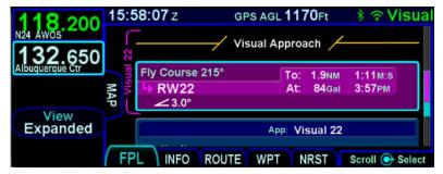
Selection of a base or downwind entry adds no additional legs to the flight plan. However, to aid in situational awareness, the entry is shown on the map using dashed lines that intercept the final approach leg, as shown below:
