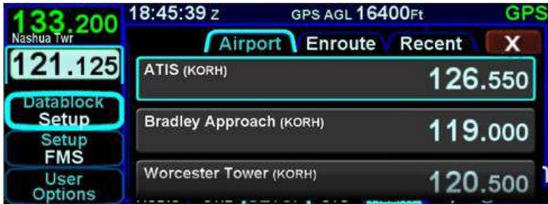
The selected tab can be changed by rotating the right outer knob or by touching the desired tab. The airport and enroute tabs only populate when there is a GPS position.
