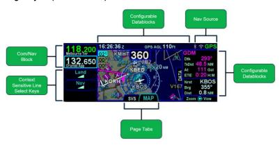
Each page has a number of associated tabs. To select a tab using the page key, press the left or right side of the key to move left or right, respectively, through the tabs until the desired tab is selected. To select a tab using the touchscreen, just touch the desired tab. When switching pages, the last tab selected on a page will be displayed when you return to that page.
