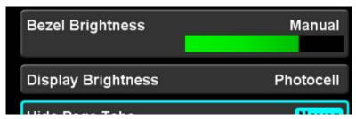
Depending on how the installer configured the brightness controls at time of installation, the "Photocell" setting will typically revert to the dimming bus setting in low ambient light conditions.
