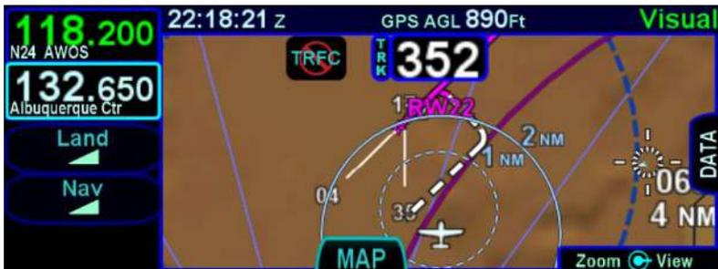
When flying a visual approach, lateral deviations are provided to the final approach course. Advisory vertical deviations are also provided once the aircraft track is at most 90 degrees to the final approach course. Therefore, on a downwind entry the VDI will remain flagged until the aircraft completes the turn to base. Vertical deviations will be provided until the aircraft is within 0.1 nautical miles of the runway threshold.
