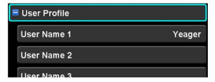
User profiles can be useful in situations where an aircraft is shared among several pilots and each pilot has different preferences for viewing data on and interacting with the IFD. In scenarios where an aircraft is always flown by the same pilot, it may be useful to define a profile for VFR flights and another profile for IFR flights. From the factory, a single user profile named "User-1" is defined.
