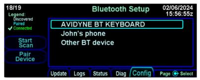
Use the right knob so that the cursor surrounds the keyboard device to be paired. Then, press the "Pair Device" LSK. What happens next is dependent on the Bluetooth version used by the keyboard. Early versions of the keyboard require entry of a code for pairing. Later versions do not. The IFD recognizes the kind of keyboard and reacts accordingly.
