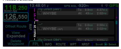
In the "Compact" view, when the flight plan is inactive, each row represents a procedure in the flight plan. Therefore, airways, departures, arrivals, and approaches all take up only a single row. When the flight plan is active, however, the procedure that contains the active leg is always expanded. The compact view is useful for viewing flight plans in a format that more closely resembles a clearance.
