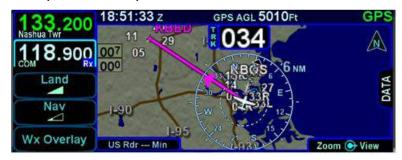
North Up can be either Magnetic North or True North depending on the "Bearing Reference" selection on the Setup Page.
