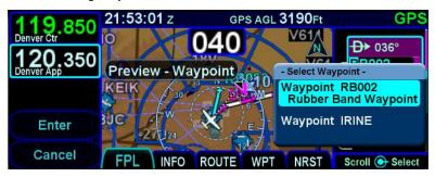
When a dropdown selection is made, the selected waypoint is inserted into the flight plan. Using the split MAP-FPL view allows the changes to the flight plan to be observed while rubber banding.
