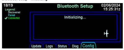
During the time that the IFD is initializing its Bluetooth interface, the Bluetooth page will appear as shown above with the aircraft symbol moving left to right across the page. The legend in the upper left corner of the page is for reference only. It does not reflect the status of Bluetooth pairing for any device.
