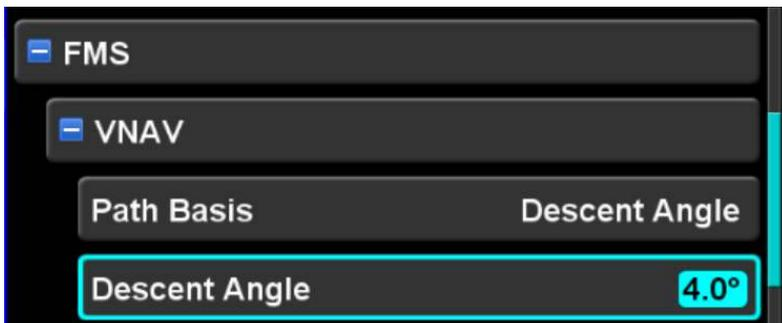
Using the enroute VNAV altitude target and the associated waypoint, the IFD will project that angle along the flight path all the way to the current aircraft altitude. That point is depicted on the map as a green circle labeled "TOD" (top-of-descent). When enroute VNAV is allowed and the aircraft reaches the TOD point, the IFD will automatically commence enroute VNAV.
