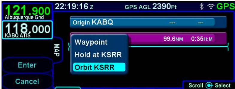
The orbit radius can range from 0.5nm to 100nm. The FMS will not actually fly to the orbit fix and instead, will fly to the point where the leg to the fix intercepts the orbit.
