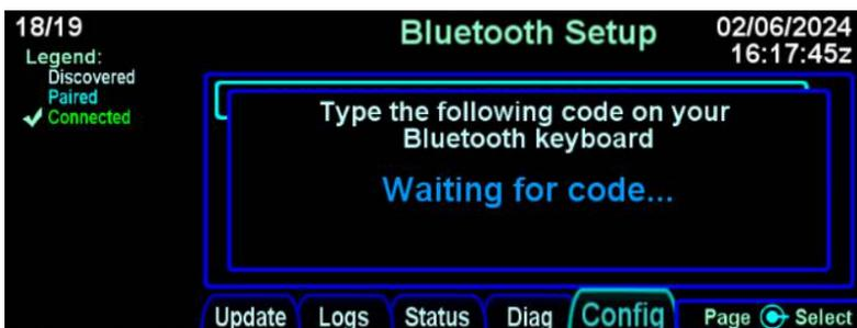
Once the code is received from the keyboard, it is displayed on the page with instructions as illustrated below. Enter the code using the Bluetooth keyboard and press ENTR.
