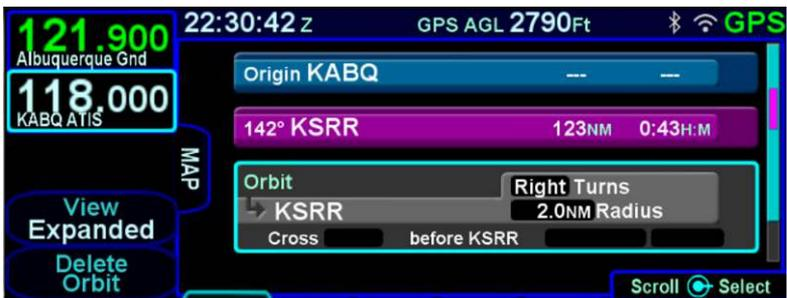
If the orbit radius is larger than the distance from the aircraft to the orbit fix, the aircraft will intercept the orbit on the extended radial between the orbit fix and the aircraft. Just like a traditional holding pattern, there is no insert cursor between a fix and a subsequent orbit. The only way to get out of an orbit is to command a Direct-To or activate a different leg. The orbit size can be changed while it is active but no path to reacquire the orbit is depicted on the map.
