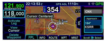
The Circular Orbit function can be enabled on the Setup Page by setting the "Patterns" field to "On".
