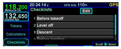
When you have finished naming the new checklist, press the "Enter" button on the keypad or push the right knob. Repeat this process for naming new checklists until all desired checklist names are created.
