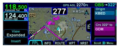
In OBS FROM (when the difference between the selected OBS course and the aircraft course to the fix is greater than or equal to 90°), the system will activate the reciprocal course away from the station with guidance away FROM the fix. The previously active TO leg will change to white and remain in pivot. The assumption here is that you will want to fly the leg on the 180° plane between
