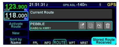
If the receiving IFD already contains the route, the receiving IFD holds the received route in a "pending" state and displays an advisory indicating the same. To store the route, switch to the ROUTE tab and press ENTR, press the Enter LSK, or touch the green confirmation box. To discard the received route and leave the existing route unchanged, press the CLR key or the Cancel LSK.
