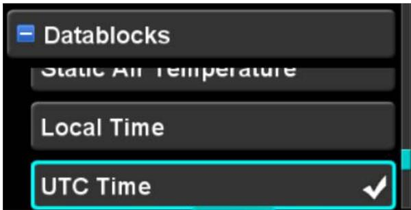
Once the datablocks category is expanded, the operation of the right knob is slightly different than the normal Setup Page operation. The outer knob selects the datablock “slot” to be affected. The inner knob selects the datablock that is to be displayed in the selected slot. The selected slot is shown with a blue background (except for the VLOC radio block). The selected datablock is shown with the typical cyan cursor surrounding the item.
