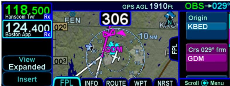
OBS mode can be used to create a user-defined course into a waypoint/fix or an airfield. Once in OBS mode, use the course knob to set the desired inbound course to the fix or airfield. All guidance, including that sent to an autopilot, will now be with respect to that user-defined course.
