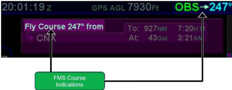
The FMS Course function will always be armed (i.e. it will always intercept the flight plan) in a To intercept. If the airplane is in a From course, it will intercept only if the dialed course trajectory intercepts the flight plan. If the dialed course does not intercept the flight plan, the airplane will fly that course indefinitely.
