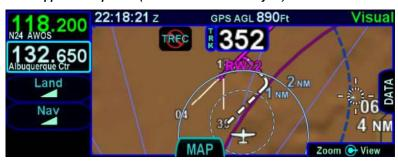
When flying a visual approach, lateral deviations are provided to the final approach course. Advisory vertical deviations are also provided once the aircraft track is at most 90 degrees to the final approach course. Therefore, on a downwind entry the VDI will remain flagged until the aircraft completes the turn to base. Vertical deviations will be provided until the aircraft is within 0.1 nautical miles of the runway threshold.
