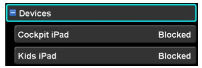
When a device is blocked, the pilot must take action to set the communication policy for that device. If the device is trusted and will always be under control of the pilot, setting the connection policy to "Always" is appropriate. If the pilot prefers to specifically determine whether that device should be allowed on every connection attempt, the connection policy should be set to "Once". If this device is not known to the pilot, the connection policy should be set to "Never".
