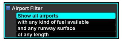
Each of the settings is edited using the typical controls for enumerated items once the filter item has been expanded.
