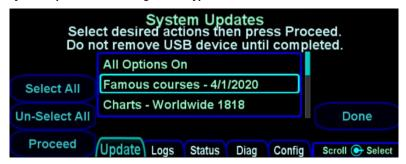
When uploading user waypoints from a CSV file, it is important to remember that the set of user waypoints in the CSV file will completely replace the set of user waypoints in the IFD.
