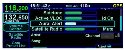
Touch control can also be used to make all those adjustments (e.g. selecting a row by touching, changing a volume level by touch dragging the bar, turning squelch on/off by tapping the correct area on the display, etc).
