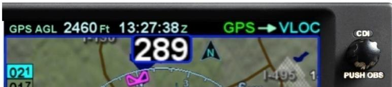
The IFD410 nav source button is similar to the nav source knob, except that it toggles only between GPS based navigation to the flight plan and an OBS course to the active waypoint.
