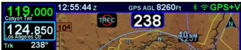
Vertical deviations can be displayed on some external indicators and will continue to be provided along the descent until the target altitude has been reached. During descent, if the aircraft deviates from the intended flight path by more than 2nm or if the aircraft course deviates by more than 45 degrees from the desired track, enroute VNAV deviations will be flagged until the aircraft resumes flight along the flight plan.
