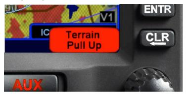
Pressing the "CLR" bezel key or touching the message bar on the display will acknowledge the message, causing the message bar for that alert to disappear. Note that acknowledging the message does not eliminate the condition that caused the alert. However, some alert messages are issued in response to an event, and acknowledging the alert effectively clears the condition.
