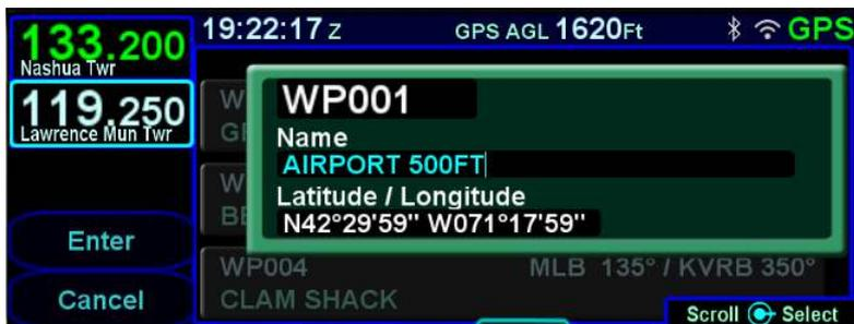
When used in a flight plan, the user-defined airport will display as an airfield with no known runway orientation.
