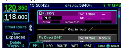
When the active leg is part of an arrival or an approach and an offpath direct-to is performed, the direct-to will be inserted after the end of the missed approach or after the destination if there is no associated missed approach. When the active leg is part of a
