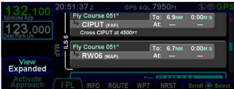
In expanded view, displayed to the right of the “to” field is a set of statistics for the leg, arranged in two lines. The first line contains the distance and time remaining on that leg (i.e. the remaining leg length and the ETE). The second line contains predicted fuel remaining (if equipped) and time (i.e. ETA) when the aircraft reaches the end of the leg.
