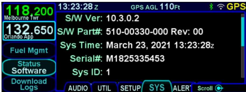
When the aircraft is not airborne, the Software Status Page will also show a “Download Logs” LSK. Pressing that LSK will put the IFD into Maintenance Mode where the datalogs can be downloaded (see page 6-32 for instructions).
