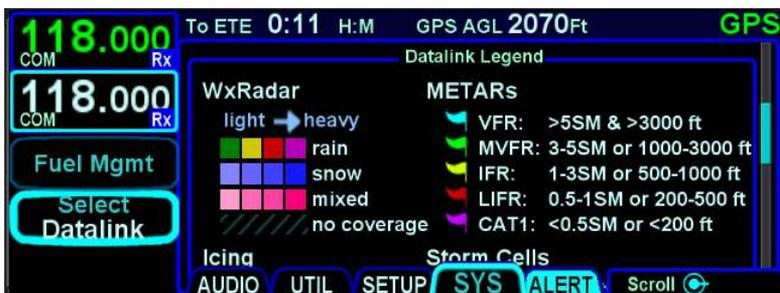
At large map ranges beyond 250nm from the aircraft, small areas of high-intensity radar returns may not be displayed; instead, larger areas of surrounding lower-intensity radar returns will be shown.
