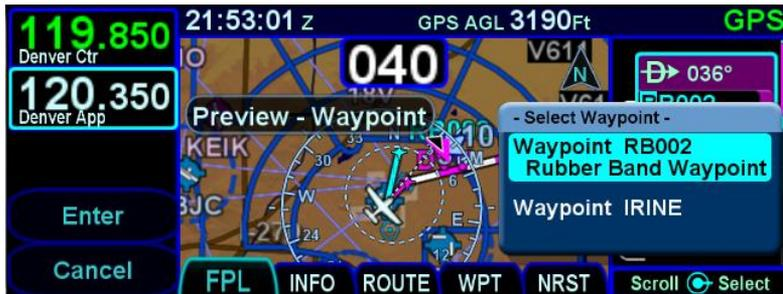
When a dropdown selection is made, the selected waypoint is inserted into the flight plan. Using the split MAP-FPL view allows the changes to the flight plan to be observed while rubber banding.
