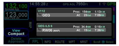
When a row represents an entire procedure, the layout is similar to that of a leg, but the "via" field contains the name of the procedure and the statistics are cumulative, covering all legs in the procedure.
