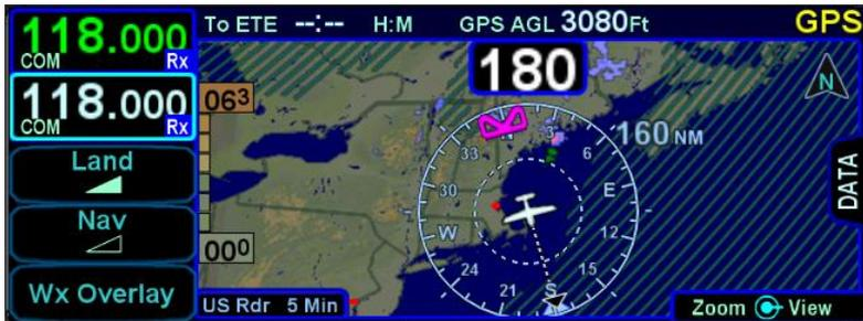
CONUS weather radar data appears noticeably coarser than subscription datalink service data and ADS-B Regional data. This is due to the lower resolution of the source data.
