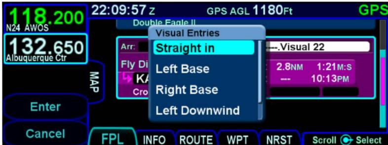
A visual approach consists of a single flight plan leg aligned with the runway heading terminating at the runway threshold. Altitude constraints cannot be entered on the visual approach leg. The area typically used to display altitude constraints is instead used to show the glideslope angle associated with the visual approach.
