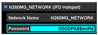
The IFD enforces the industry recommended minimum password length of 8 characters. As the field is being edited, if less than 8 characters have been entered, the IFD will ignore actions to complete the edit (e.g. **pressing the ENTR button will have no effect**). The edit can be aborted by pressing CLR.
