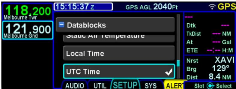
In order to change the datablock selected in a given slot, first turn the outer knob or touch to move the cursor to the desired slot. Then, use the inner knob or touch to select the datablock item to be displayed. Then, press the knob button or touch the datablock again to place it into the selected slot.
