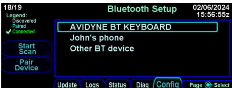
Use the right knob so that the cursor surrounds the keyboard device to be paired. Then, press the “Pair Device” LSK. What happens next is dependent on the Bluetooth version used by the keyboard. Early versions of the keyboard require entry of a code for pairing. Later versions do not. The IFD recognizes the kind of keyboard and reacts accordingly.
