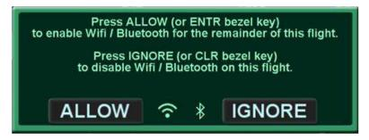
To disconnect Wi-Fi and Bluetooth interfaces, either touch "Ignore" or press the CLR button. From that point on, the IFD will not connect with devices over those two interfaces.
