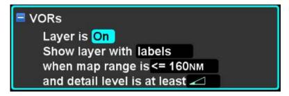
Like the airport filter, the layout and wording of conditions within a map layer is designed to make the set of conditions read like a sentence. The sentence is structured to clearly specify the set of conditions that must be met in order for items in the layer to be shown. Each of the possible criteria is described as follows.
