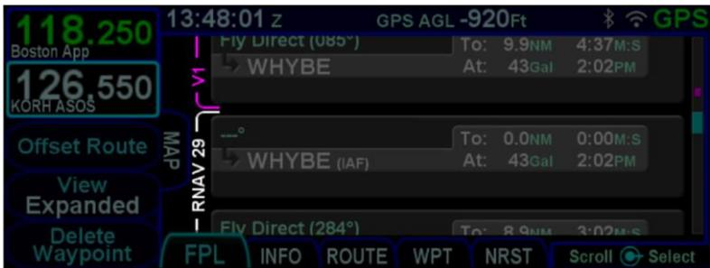
In the "Compact" view, when the flight plan is inactive, each row represents a procedure in the flight plan. Therefore, airways, departures, arrivals, and approaches all take up only a single row. When the flight plan is active, however, the procedure that contains the active leg is always expanded. The compact view is useful for viewing flight plans in a format that more closely resembles a clearance.
