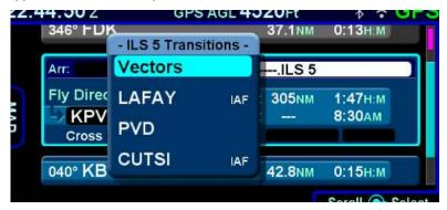
After having selected the procedure, including related transitions, the legs will be inserted into the flight plan and the corresponding destination airport field will contain the name of the procedure that was just inserted.
