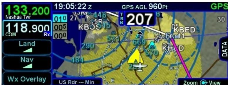
Terrain Awareness coloring can be triggered by terrain within a 10nm radius of the aircraft and is displayed as follows, depending upon the installation:
