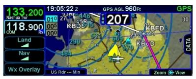
Terrain Awareness coloring can be triggered by terrain within a 10nm radius of the aircraft and is displayed as follows, depending upon the installation:
