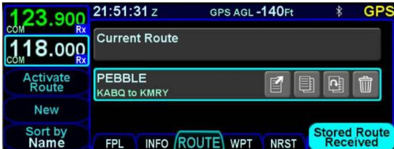
If the receiving IFD already contains the route, the receiving IFD holds the received route in a “pending” state and displays an advisory indicating the same. To store the route, switch to the ROUTE tab and press ENTR, press the Enter LSK, or touch the green confirmation box. To discard the received route and leave the existing route unchanged, press the CLR key or the Cancel LSK.
