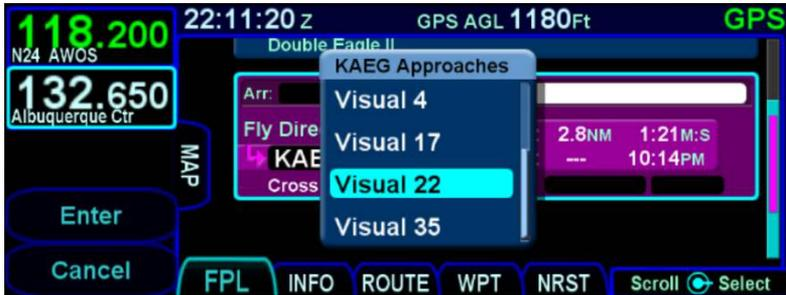
Once a visual approach has been selected, the familiar transition dropdown will appear. The dropdown contains selections for a straight-in approach and for base and downwind pattern entries using both left and right turns, as illustrated below.
