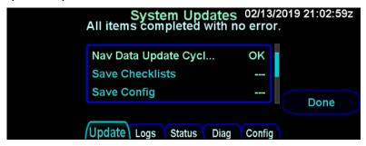
When all loading operations have been completed, press the "Done" LSK to restart the IFD in flight mode. Remove the USB flash drive and store it in a safe place. If the USB flash drive is inadvertently left in the USB port during flight mode, there will be no adverse affect as the USB flash drive is ignored during flight mode.
