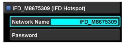
Entry of a new network name will also be reflected on the IFD LAN item (i.e. the header).
