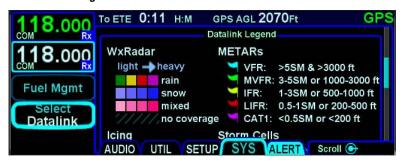
At large map ranges beyond 250nm from the aircraft, small areas of high-intensity radar returns may not be displayed; instead, larger areas of surrounding lower-intensity radar returns will be shown.
