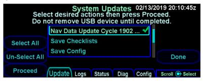
Once the set of items to be loaded has been selected, press the Proceed LSK to start the load.
