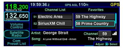
The page is divided into three parts. The left side of the page is a full channel list of all available satellite radio channels. The right side of the page is a numbered list titled "Favorites" and represents the satellite radio channels that have been programmed into a preset list for faster access. The bottom of the page contains a datablock indicating the artist, song, channel name and number, audio signal strength and a Quick Go To link to enter in a desired satellite audio channel.
