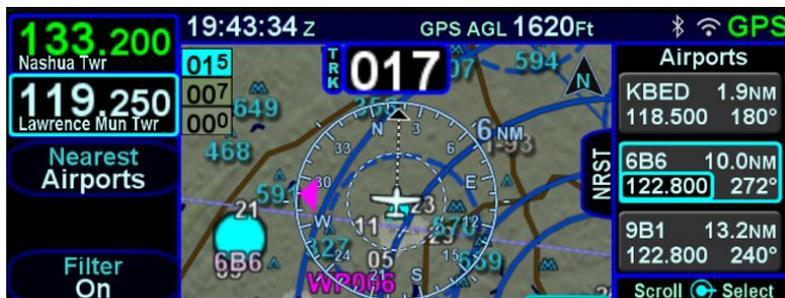
When using the split view, the facility associated with the row that is highlighted in the Nearest list will also be highlighted with a cyan circle on the map (see 6B6 in the split page view above)
