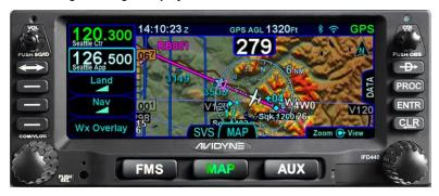
Supplemental IFD functions include a moving-map, flight management system (FMS), checklists, and a number of timer and calculator types of utilities. Optional IFD functions include control and display of remote transponders. The system includes terrain alerting as well as an option for HTAWS.
