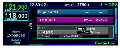
If the orbit radius is larger than the distance from the aircraft to the orbit fix, the aircraft will intercept the orbit on the extended radial between the orbit fix and the aircraft. Just like a traditional holding pattern, there is no insert cursor between a fix and a subsequent orbit. The only way to get out of an orbit is to command a Direct-To or activate a different leg. The orbit size can be changed while it is active but no path to reacquire the orbit is depicted on the map.
