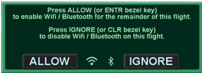
To disconnect Wi-Fi and Bluetooth interfaces, either touch "Ignore" or press the CLR button. From that point on, the IFD will not connect with devices over those two interfaces.
