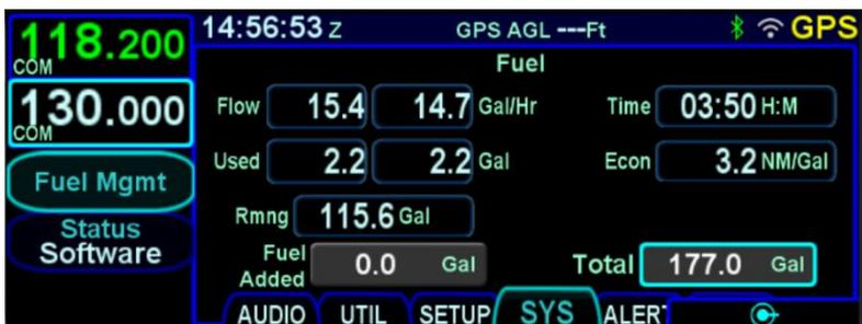
If the fuel flow system is not capable of reporting the amount of fuel remaining (i.e. does not have a totalizer), then the IFD will present two controls allowing the fuel quantity to be manually adjusted.
