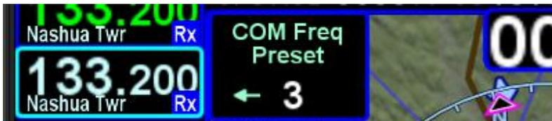
The swap frequency button performs the same action as pressing the Frequency Swap button on the bezel, including holding it down to tune the emergency frequency.
