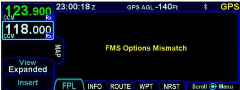
If the IFDs have mismatched software versions, sensor and control data (e.g. weather, traffic, fuel, volumes, keyboard convenience mode, etc.) will not be shared between the IFDs.
