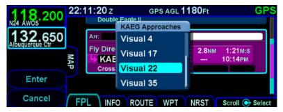
Once a visual approach has been selected, the familiar transition dropdown will appear. The dropdown contains selections for a straight-in approach and for base and downwind pattern entries using both left and right turns, as illustrated below.
