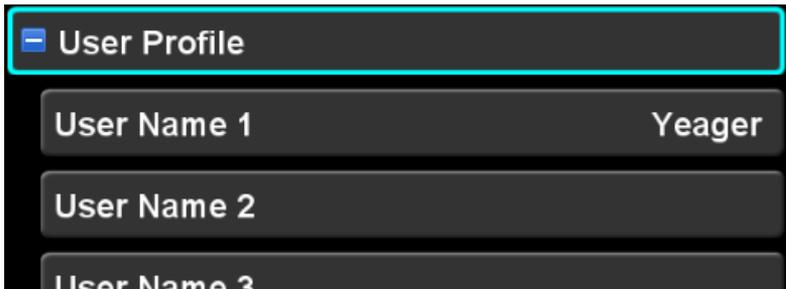
User profiles can be useful in situations where an aircraft is shared among several pilots and each pilot has different preferences for viewing data on and interacting with the IFD. In scenarios where an aircraft is always flown by the same pilot, it may be useful to define a profile for VFR flights and another profile for IFR flights. From the factory, a single user profile named “User-1” is defined.
