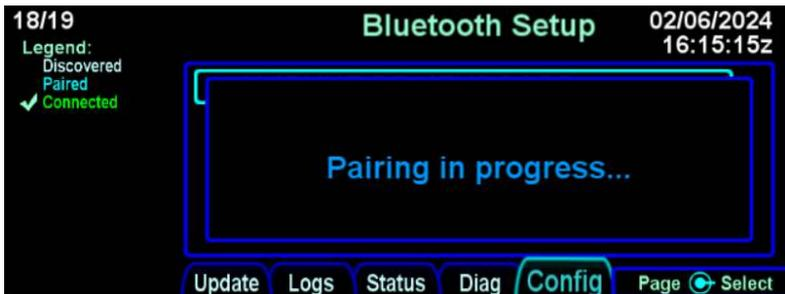
Regardless of whether a code entry was required, if the pairing process is successful, the selected device is shown in green with a checkmark next to it.
