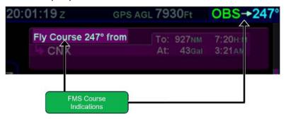
The FMS Course function will always be armed (i.e. it will always intercept the flight plan) in a To intercept. If the airplane is in a From course, it will intercept only if the dialed course trajectory intercepts the flight plan. If the dialed course does not intercept the flight plan, the airplane will fly that course indefinitely.
