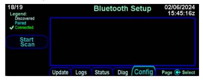
Press the Start Scan LSK to start the process of discovering available Bluetooth devices. Turn the keyboard on using the slide switch on the left side of the keyboard, then press and hold the button on the back of the keyboard. Release the button once the pairing light in the upper left corner of the keyboard starts flashing. On newer keyboards, the button must be held long enough for the light to start flashing rapidly – generally a few seconds.
