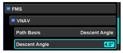
Using the enroute VNAV altitude target and the associated waypoint, the IFD will project that angle along the flight path all the way to the current aircraft altitude. That point is depicted on the map as a green circle labeled "TOD" (top-of-descent). When enroute VNAV is allowed and the aircraft reaches the TOD point, the IFD will automatically commence enroute VNAV.
