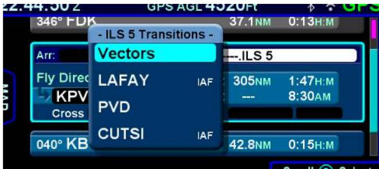
After having selected the procedure, including related transitions, the legs will be inserted into the flight plan and the corresponding destination airport field will contain the name of the procedure that was just inserted.
