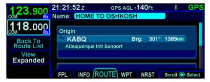
To remove a manually entered route name, move the cursor to the route name field and press the "CLR" button. At that point, the IFD will generate a name as specified above.
