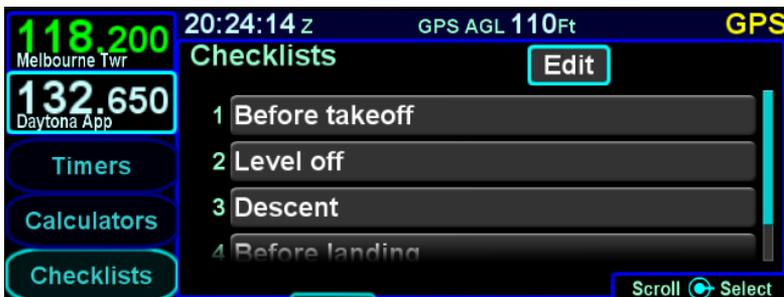
When you have finished naming the new checklist, press the “Enter” button on the keypad or push the right knob. Repeat this process for naming new checklists until all desired checklist names are created.
