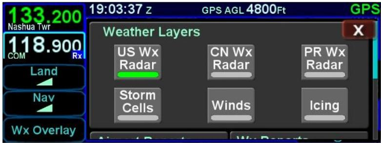
The Wx Overlay page is segmented into groupings of products. Products selected for overlay are indicated by a green lamp. Note that the products in the “Weather Layers” group are mutually exclusive. The table below represents the possible set of products available. Products that are not available due to the device type or subscription level will not be displayed as selectable choices.
