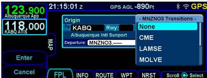
Once the enroute transition has been selected, the FMS will process runway transitions. There are departures that do not have published runway transitions. For those cases, the rest of this process is skipped and the selected procedure and enroute transition are inserted into the flight plan. Otherwise, the FMS
