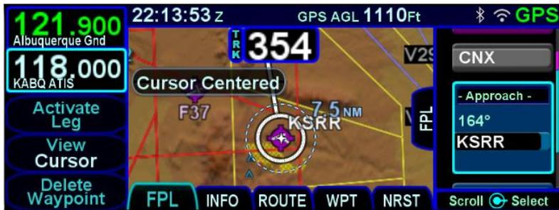
The Circular Orbit function can be enabled on the Setup Page by setting the "Patterns" field to "On".
