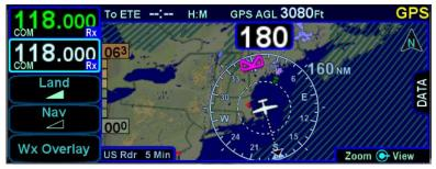
CONUS weather radar data appears noticeably coarser than subscription datalink service data and ADS-B Regional data. This is due to the lower resolution of the source data.
