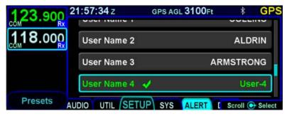
To load a different user profile into the current settings, rotate the right knob or touch to select the desired user profile, then press the "Load" LSK. If the selected user profile is the same as the
