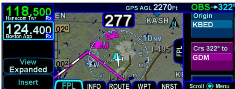
In OBS FROM (when the difference between the selected OBS course and the aircraft course to the fix is greater than or equal to  $90^\circ$ ), the system will activate the reciprocal course away from the station with guidance away FROM the fix. The previously active TO leg will change to white and remain in pivot. The assumption here is that you will want to fly the leg on the  $180^\circ$  plane between
