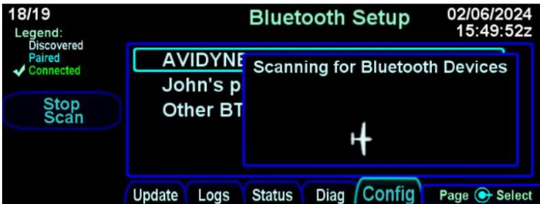
When the name of the keyboard appears, press “Stop Scan”.
