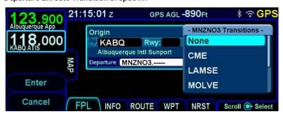
Once the enroute transition has been selected, the FMS will process runway transitions. There are departures that do not have published runway transitions. For those cases, the rest of this process is skipped and the selected procedure and enroute transition are inserted into the flight plan. Otherwise, the FMS
