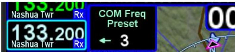
On the com preset page, a small arrow indicates which preset is tuned.
