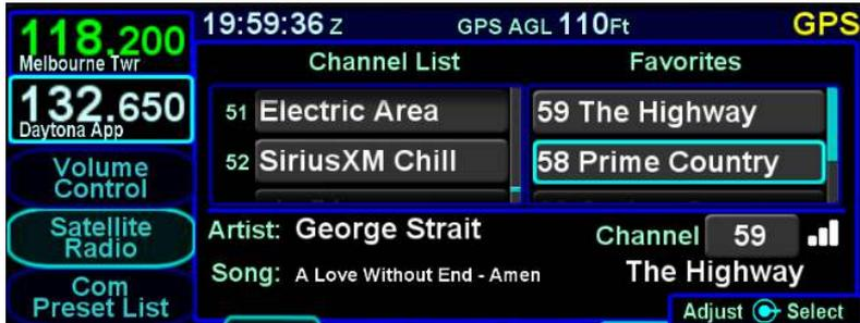
The page is divided into three parts. The left side of the page is a full channel list of all available satellite radio channels. The right side of the page is a numbered list titled “Favorites” and represents the satellite radio channels that have been programmed into a preset list for faster access. The bottom of the page contains a datablock indicating the artist, song, channel name and number, audio signal strength and a Quick Go To link to enter in a desired satellite audio channel.
