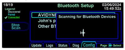
When the name of the keyboard appears, press "Stop Scan".
