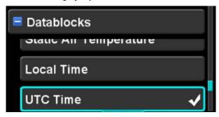
Once the datablocks category is expanded, the operation of the right knob is slightly different than the normal Setup Page operation. The outer knob selects the datablock "slot" to be affected. The inner knob selects the datablock that is to be displayed in the selected slot. The selected slot is shown with a blue background (except for the VLOC radio block). The selected datablock is shown with the typical cyan cursor surrounding the item.
