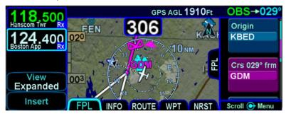
OBS mode can be used to create a user-defined course into a waypoint/fix or an airfield. Once in OBS mode, use the course knob to set the desired inbound course to the fix or airfield. All guidance, including that sent to an autopilot, will now be with respect to that user-defined course.
