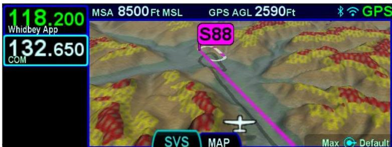
Any traffic in the scene will cast a shadow on the ground to help with judging distance and relative closure rate.
