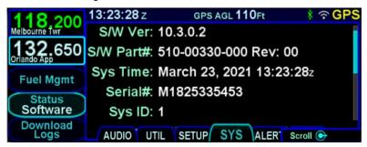
When the aircraft is not airborne, the Software Status Page will also show a "Download Logs" LSK. Pressing that LSK will put the IFD into Maintenance Mode where the datalogs can be downloaded (see page 6-32 for instructions).
