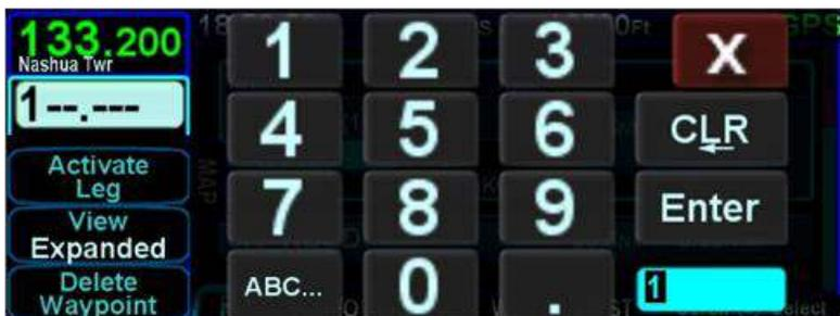
Each keyboard has an associated scratchpad which shows the entry in progress. In most cases, the scratchpad content is formatted to include characters that may not have been entered. For instance, during a distance entry of “123”, the scratchpad may contain “123.0 NM”.
