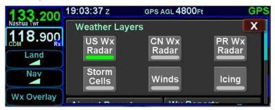
The Wx Overlay page is segmented into groupings of products. Products selected for overlay are indicated by a green lamp. Note that the products in the "Weather Layers" group are mutually exclusive. The table below represents the possible set of products available. Products that are not available due to the device type or subscription level will not be displayed as selectable choices.
