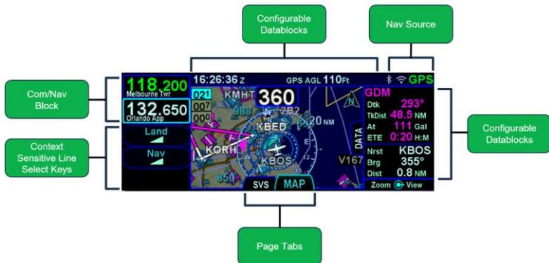
Each page has a number of associated tabs. To select a tab using the page key, press the left or right side of the key to move left or right, respectively, through the tabs until the desired tab is selected. To select a tab using the touchscreen, just touch the desired tab. When switching pages, the last tab selected on a page will be displayed when you return to that page.
