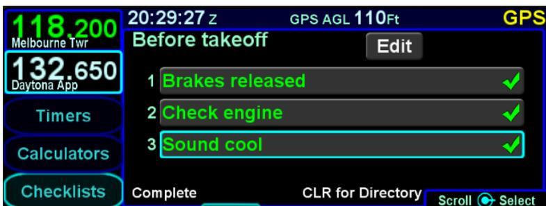
If a step inadvertently has been checked off as accomplished, it can be unchecked by selecting the step (touch it or use the bottom right knob) and then touching it a second time or pushing the knob to remove the checkmark. This will also toggle the “Checklist Complete” text back to “Checklist Not Completed”.
