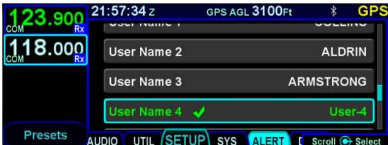
To load a different user profile into the current settings, rotate the right knob or touch to select the desired user profile, then press the “Load” LSK. If the selected user profile is the same as the
