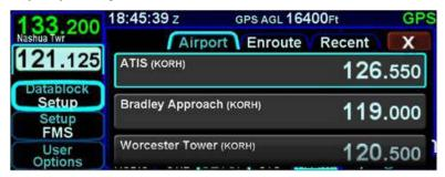
The selected tab can be changed by rotating the right outer knob or by touching the desired tab. The airport and enroute tabs only populate when there is a GPS position.
