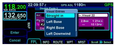
A visual approach consists of a single flight plan leg aligned with the runway heading terminating at the runway threshold. Altitude constraints cannot be entered on the visual approach leg. The area typically used to display altitude constraints is instead used to show the glideslope angle associated with the visual approach.
