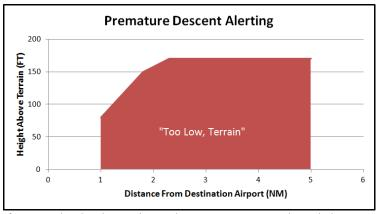
If a PDA alert has been triggered, a CAS message and aural alert "Too Low Terrain" will be issued and repeat every 6 seconds until it is acknowledged, or the condition is no longer true. For the condition to no longer be true, the aircraft must clear the alerting altitude by 100 feet. So, for example, if the aircraft is 4 NM away from the
