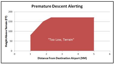
If a PDA alert has been triggered, a CAS message and aural alert "Too Low Terrain" will be issued and repeat every 6 seconds until it is acknowledged, or the condition is no longer true. For the condition to no longer be true, the aircraft must clear the alerting altitude by 100 feet. So, for example, if the aircraft is 4 NM away from the airport and descended to 150 feet AGL, a climb to 270 feet AGL must be completed to clear the condition.
