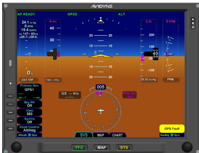
Figure 4 Loss of Dual GPS
