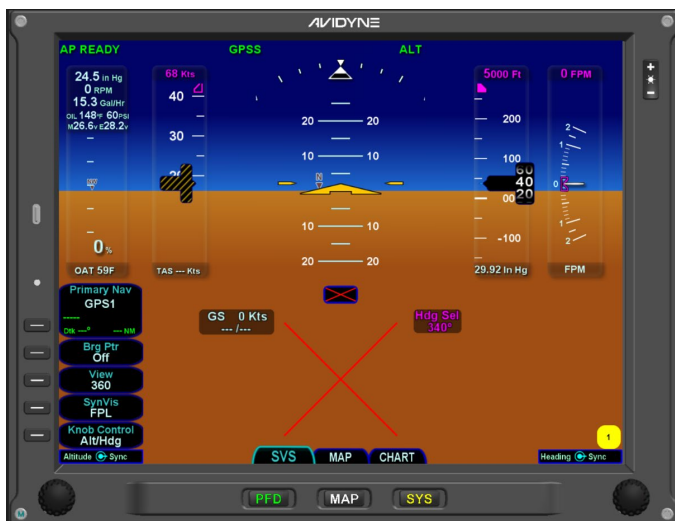
Figure 7 Loss of Single Magnetometer
