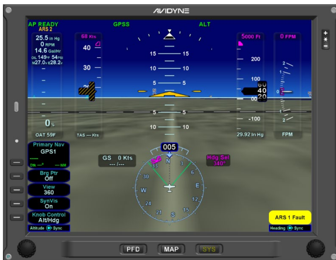
Figure 6 Loss of Single ADC
