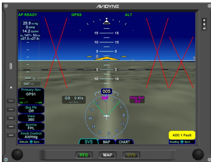
Figure 2 Loss of Single ADC
