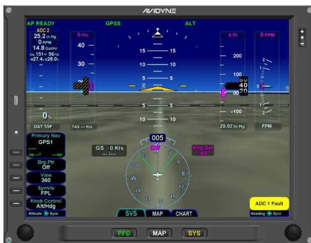
Figure 5 Loss of Single ADC
