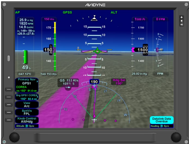
Figure 8 - Avidyne Vantage12 700-00212-010 Primary Flight Display
