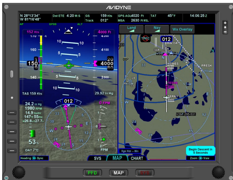
Figure 9 MFD in PFD Reversionary Mode
