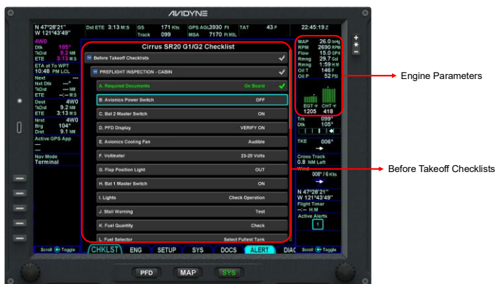
Figure 4-7 Engine Datablock beside checklist
