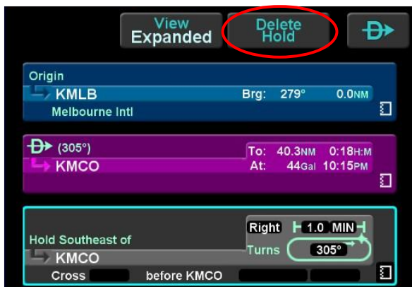
Figure 6-12 Deleting a holding pattern
