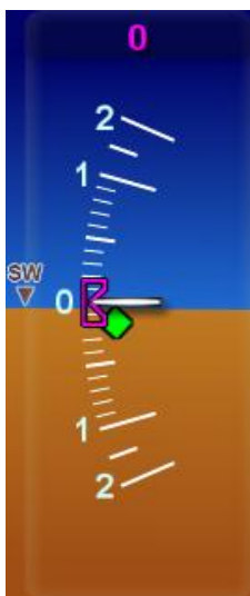
Figure 7-2 Vertical Speed Required (green diamond)
