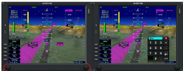
Figure 4-9 Setting the Autopilot Bugs
