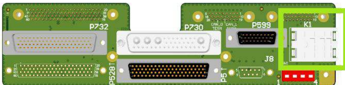
Figure A-14: Vantage12 PFD EZ Adapter K1 Socket Location
