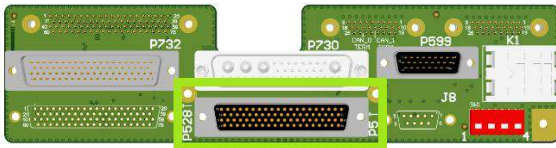
Figure A-10: Vantage12 PFD EZ Adapter P5 Connector Location and Pinout
