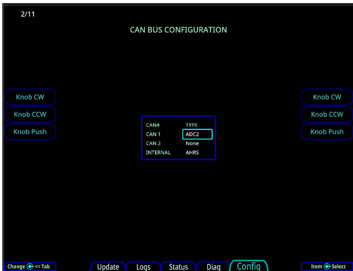
Figure 5-13: MFD CAN Bus Configuration Page
