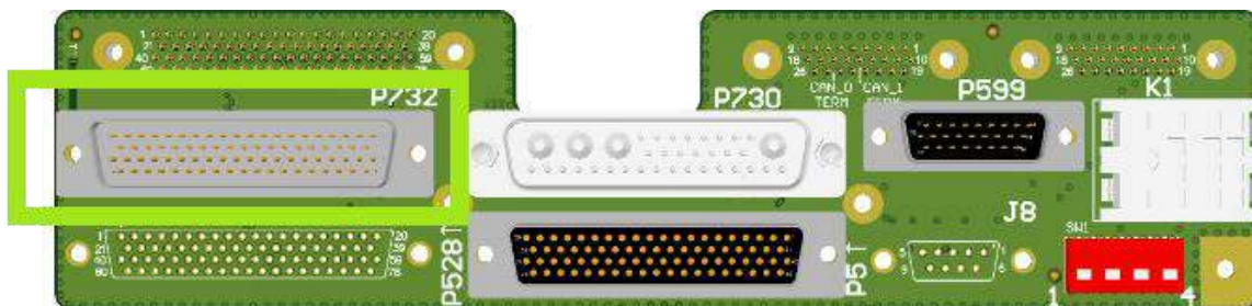
Figure A-12: Vantage12 PFD EZ Adapter J732 Connector Location and Pinout
