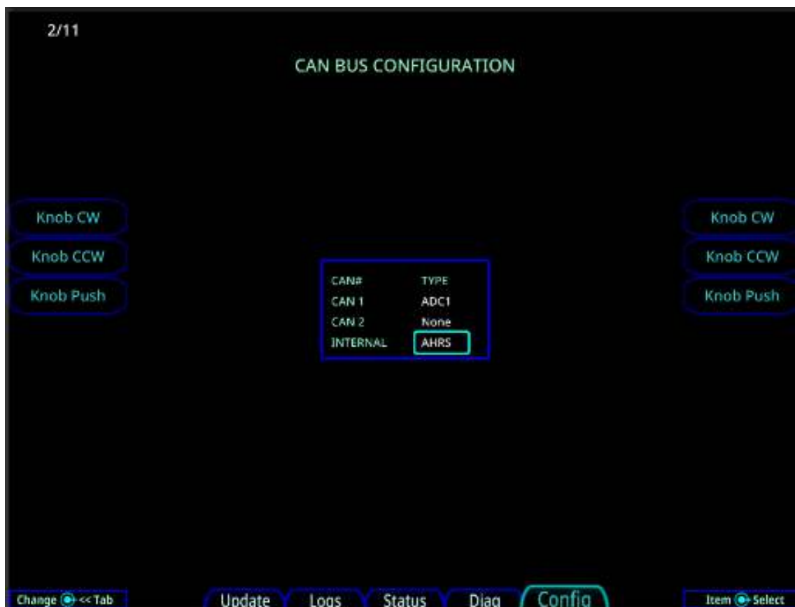
Figure 5-8: PFD CAN Bus Config Page
