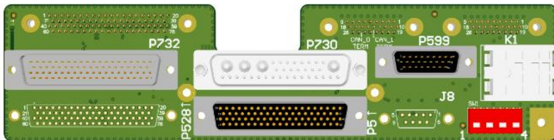
Figure A-5: Vantage12 PFD EZ Adapter Bottom View
