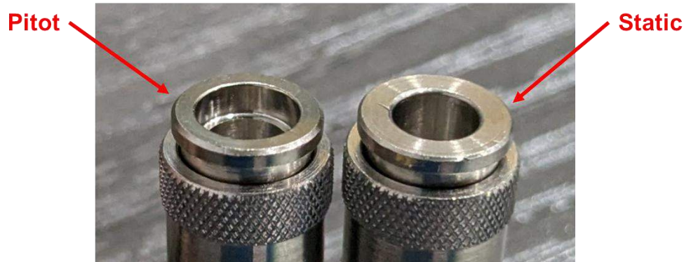
Figure 4-7: ADC Connector Keying
