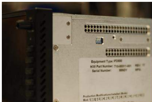
Figure 5-2: IFD Chassis ID Setting
