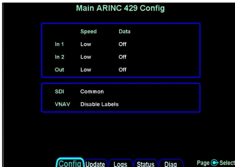
Figure 5-3: IFD Main ARINC429 Configuration Page
