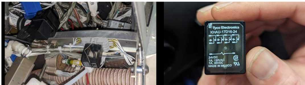
Figure 4-18: P735 Fail Safe Relay and Location
