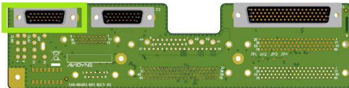
Figure A-9: Vantage12 PFD EZ Adapter P3 Connector Location and Pinout – not used
