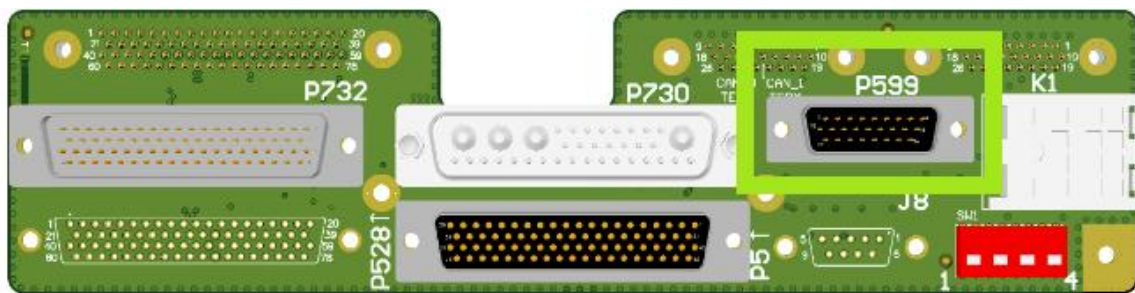
Figure A-13: Vantage12 PFD EZ Adapter P1401/P599 Connector Location and Pinout
