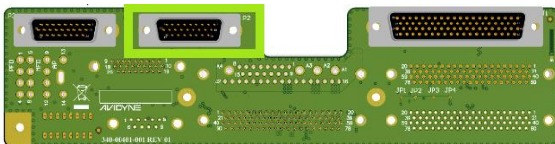
Figure A-8: Vantage12 PFD EZ Adapter P2 Location and Pinout
