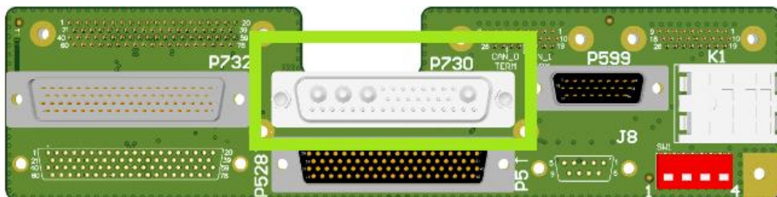
Figure A-11: Vantage12 PFD EZ Adapter P730 Connector Location and Pinout
