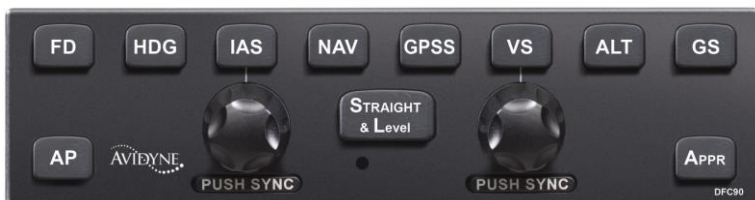
Figure 1: DFC90 Digital Flight Control System
