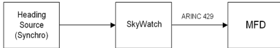
Figure 5: Heading Configuration with SkyWatch
