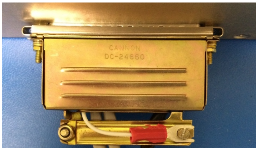
Figure 3-4: Clamp Ground Termination
