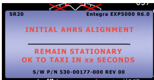
Figure 7. Entegra EXP5000 AHRS Alignment Message
