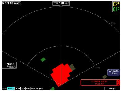
Figure 4.3 Terrain Warning Condition
