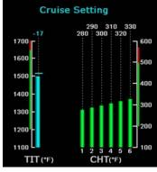
If the mixture is adjusted too far to the rich side, the EX5000 will annunciate "Too Rich." Slowly lean the mixture until the annunciation switches back to "Cruise Setting."
