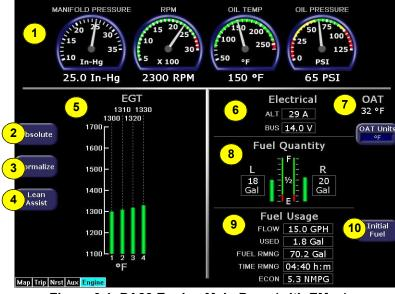
Figure 9.1 PA28 Engine Main Page (with EMax)
