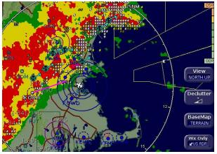
Figure 10.4 Broadcast Datalink Weather
