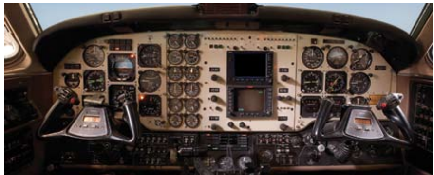
The popular King Air 200 series is a tremendous upgrade candidate for the Alliant system, replacing antiquated dials, gauges and hard-to-repair autopilots with modern all-glass flight deck.
