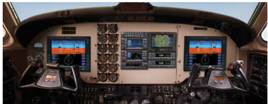
The Alliant integrated flight deck provides the state-of-the-art in situational awareness, safety, reliability, and redundancy for the King Air 200 using Avidyne's Envision integrated displays along with the S-TEC 2100 IntelliFlight autopilot.
